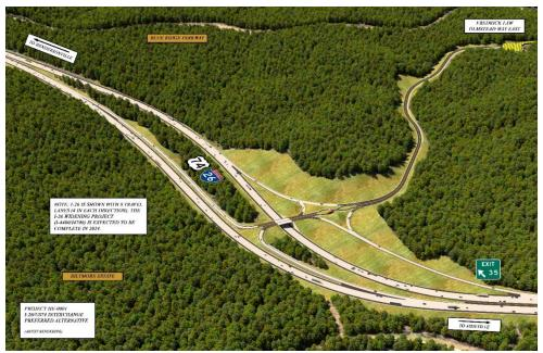
**Figure 4.** Rendering showing the new Half Diverging Diamond Interchange (DDI) (future Exit 35) and the one-half mile East Frederick Law Olmsted Way (FLOW) connector road.
